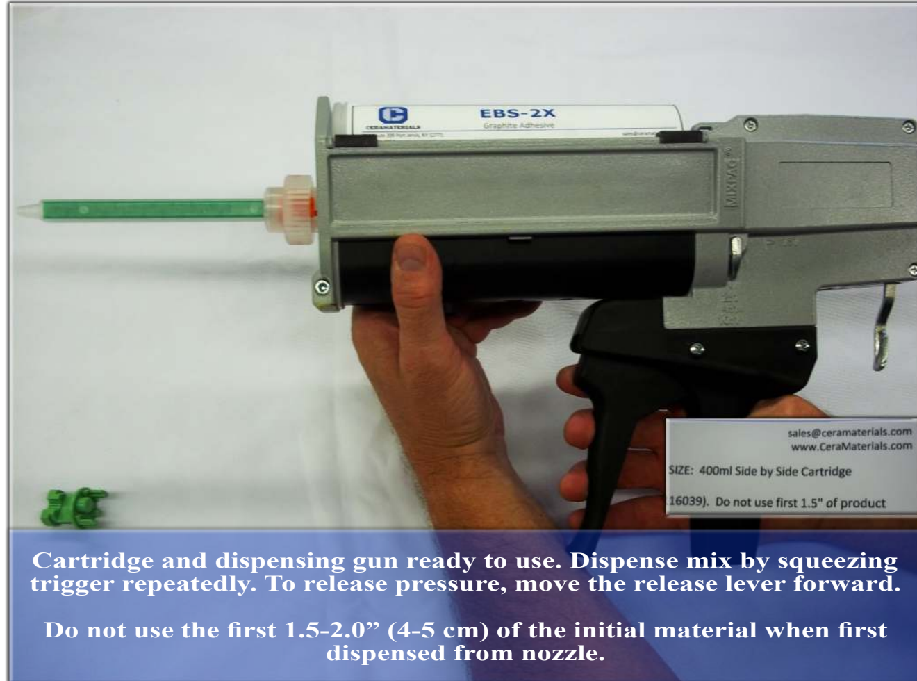
8. Place cartridge in dispensing gun, small cartridge side goes down, and push down evenly.
